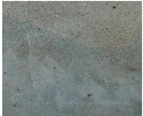
Picture shows how the top surface is removed with acid to reveal finished throwing surface. Top section of the photo shows the small granite chips exposed following single acid
